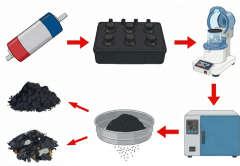
Figure 2 – Schematic illustration of electrode mass preparation process
